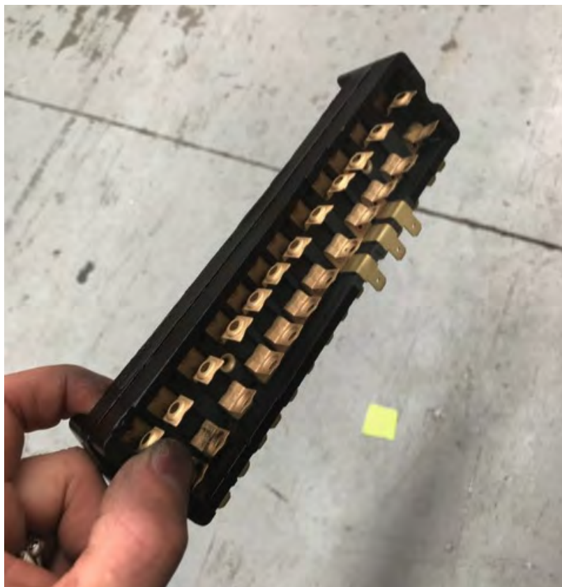
The new fuse box. They look a little different on modern cars!
